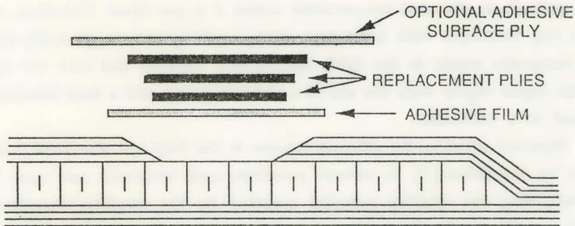
Figure 4. Flush Aerodynamic Scarf Repair for Composite Structures.
