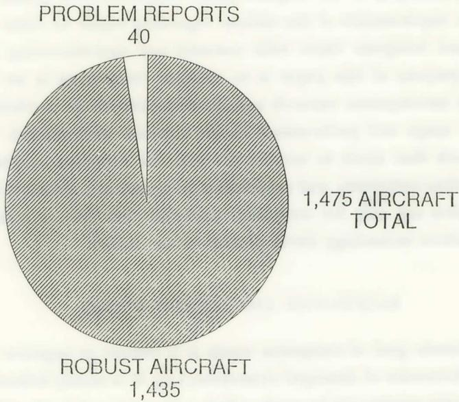
Figure 2. Survey Results of Composite Elevator Damage on Boeing B-737, 757, and 767 Aircraft.
