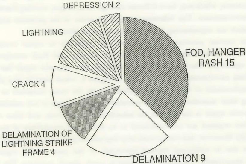
Figure 3. Type of Damage Reported on Damaged Composite Elevators as Shown in Figure 2.
