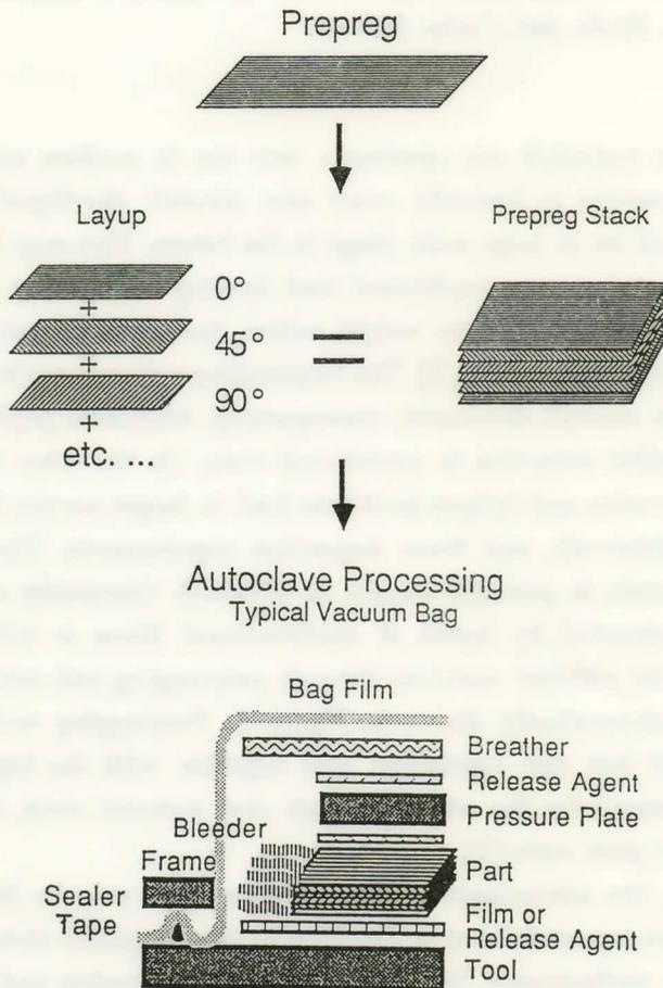
Figure 1. Laminated Structures Made of Prepreg via Vacuum Bag/Autoclave Techniques.
