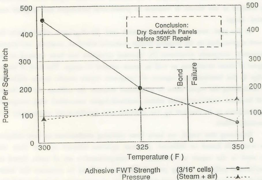
Figure 5. Calculated Honeycomb Panel Internal Pressure due to Water and Measured Adhesive Flatwise Tensile Strength as a Function of Temperature.
