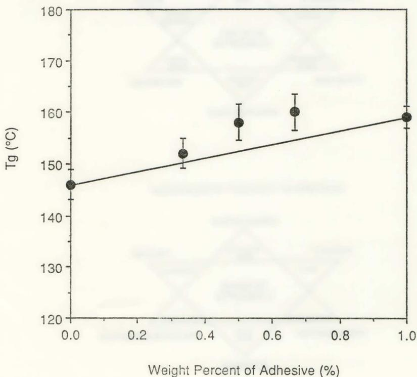
Figure 6. Glass Transition Temperature Measured by MDSC of Prepreg/Adhesive Resin Mixtures Used in Manufacturing and Repair.
