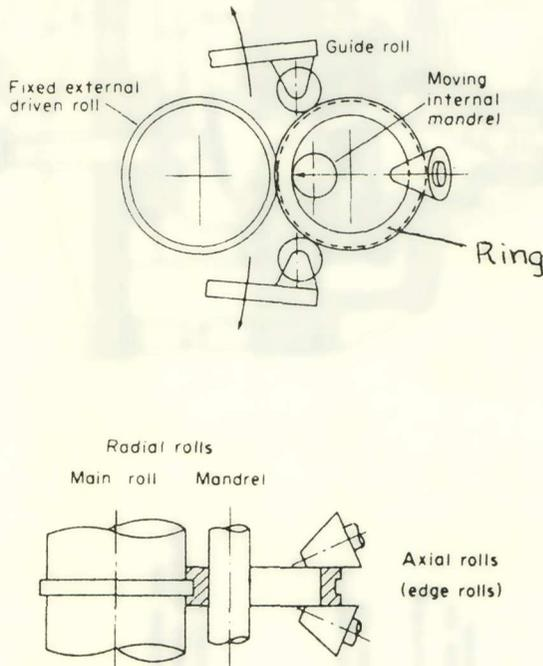
Fig. 2. The basic components of a ring-rolling mill.
