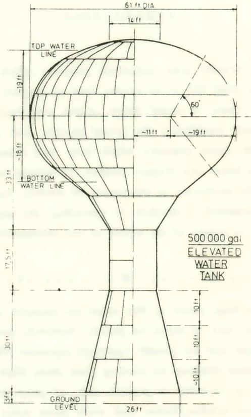
Fig. 1. A half-a-million-gallon elevated spherical watertank for erection in Saudi Arabia.
