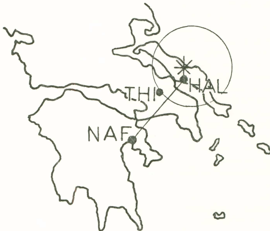
Fig. 27. Graphical determination of the epicenter from signals collected at two stations.
