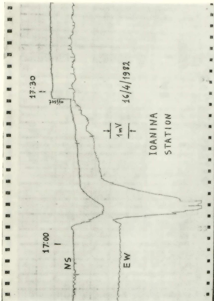
Fig. 14. Disturbance of the telluric field collected at IOA - station due to an SSC occurred on April 16th 1982.
