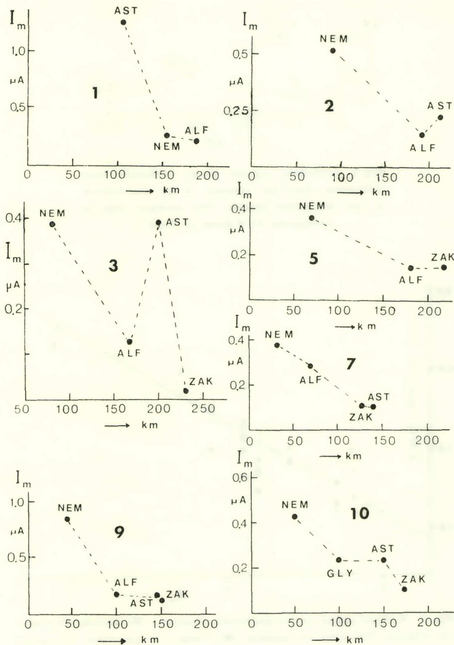
Fig 4. Coincident values of  $I_{max}$  in function of the epicentral distance. The numbers refer to earthquakes 1 to 10 given in Table I. In the plot of Nr 10 the value  $0.23 \mu A$  obtained at Glyfada ( $r = 105$  km) has been added.
