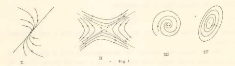
The singularities are shown in Fig. 1, where I is a «nodal stable», III a «stable spiral», IV a (neutral) center, and II a «saddle point intrincically unstable».
