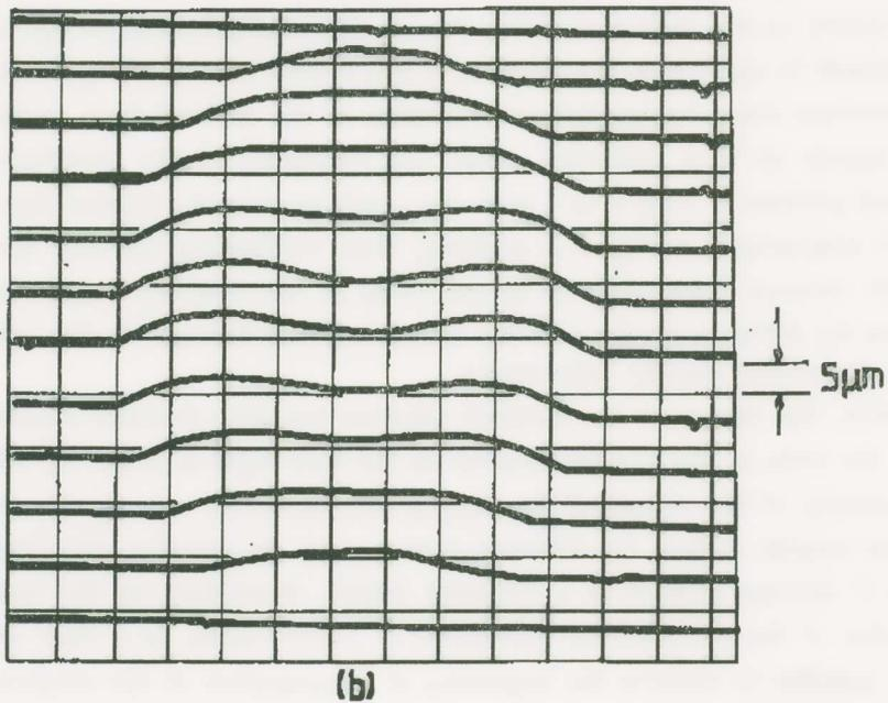
Fig. 11. Talysurf tracings of the variation of the thickness of the speckle hill by successive traverses (a) initial step (b) step with crater.
