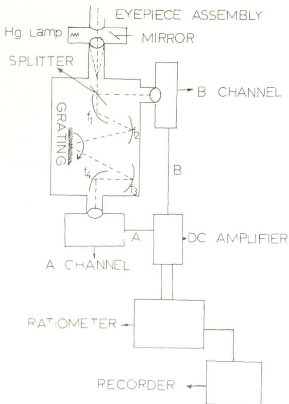
Fig 1 Schematic diagram of the photoelectric spectrum scanner.
