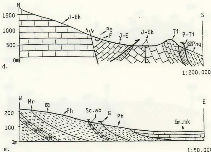
d. Crete: J - Ek = Jurassic - Eocene plattenkalk formations, Pe = Jurassic - Eocene plattenkalk formations, Pe = Peridotite, F = Flysch, J - E = Jurassic - Eocene thick bedded limestones and dolomites, Ti = Triassic laminated dolomites, P - Ti = Permian - Triassic crystalline limestones with phyllites, Phq = Permian - Triassic phyllite-quartzite (modified from I.G.S.R., 1977).
