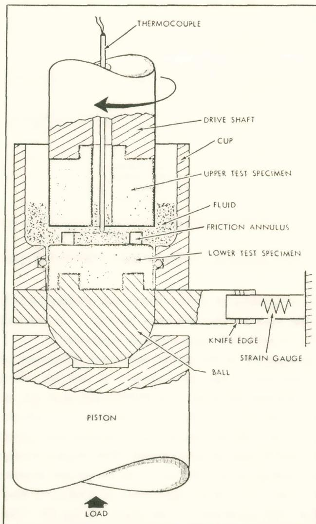
Fig. 9. Low Velocity Friction Apparatus.
