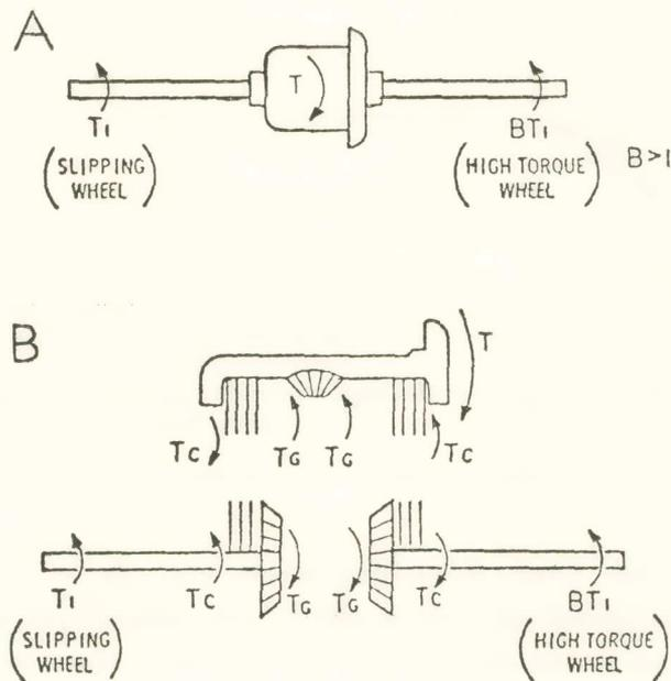
Fig. 6. Torque Diagrams: A-external
