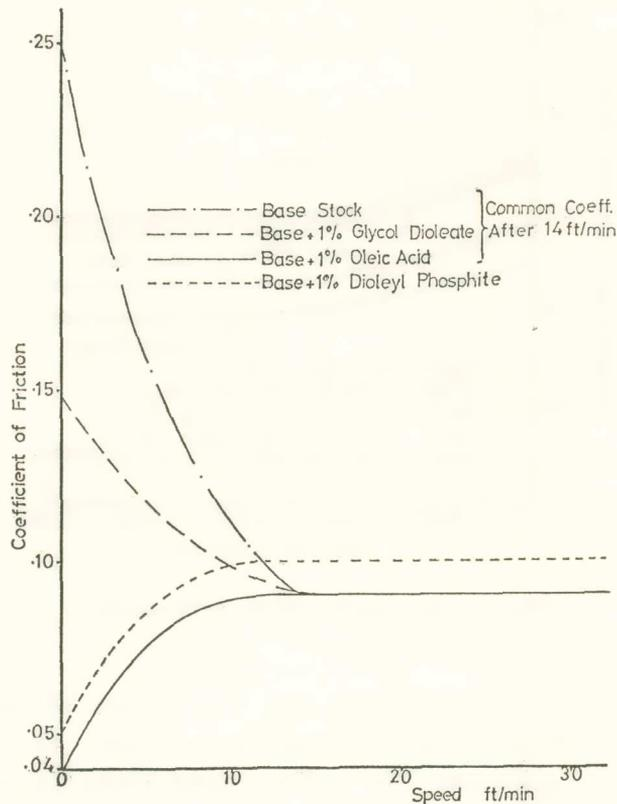
Fig. 3. Effect of Friction Modifiers on the Base Stock Friction - LVFA.
