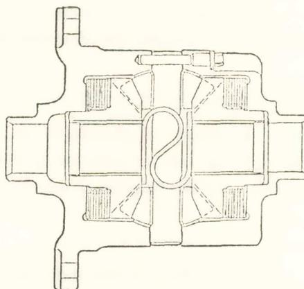
Fig. 5. Limited - Slip Differential.
