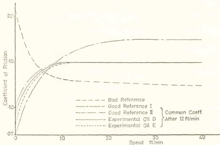
Fig. 7. LVFA Frictional Profiles of Limited-Slip Gear Oils (New).
