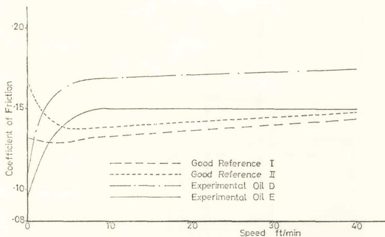
Fig. 8. LVFA Frictional Profiles of Aged Limited-Slip Gear Oils.
