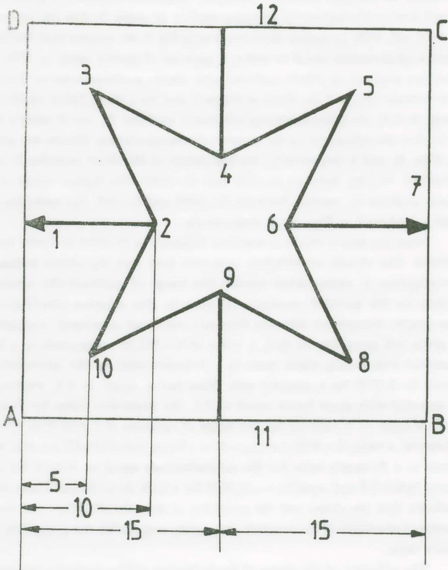
Fig. 3. A star-shaped two-dimensional beam-like cell with re-entrant corners simulating the unit cell of Fig. 2. Finite element discretization and mode numbering.
