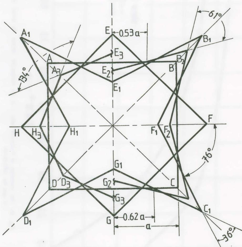
Fig. 6. Parametric investigation of five types of a star-shaped two dimensional unit cell expressed as a truss-like structure.
