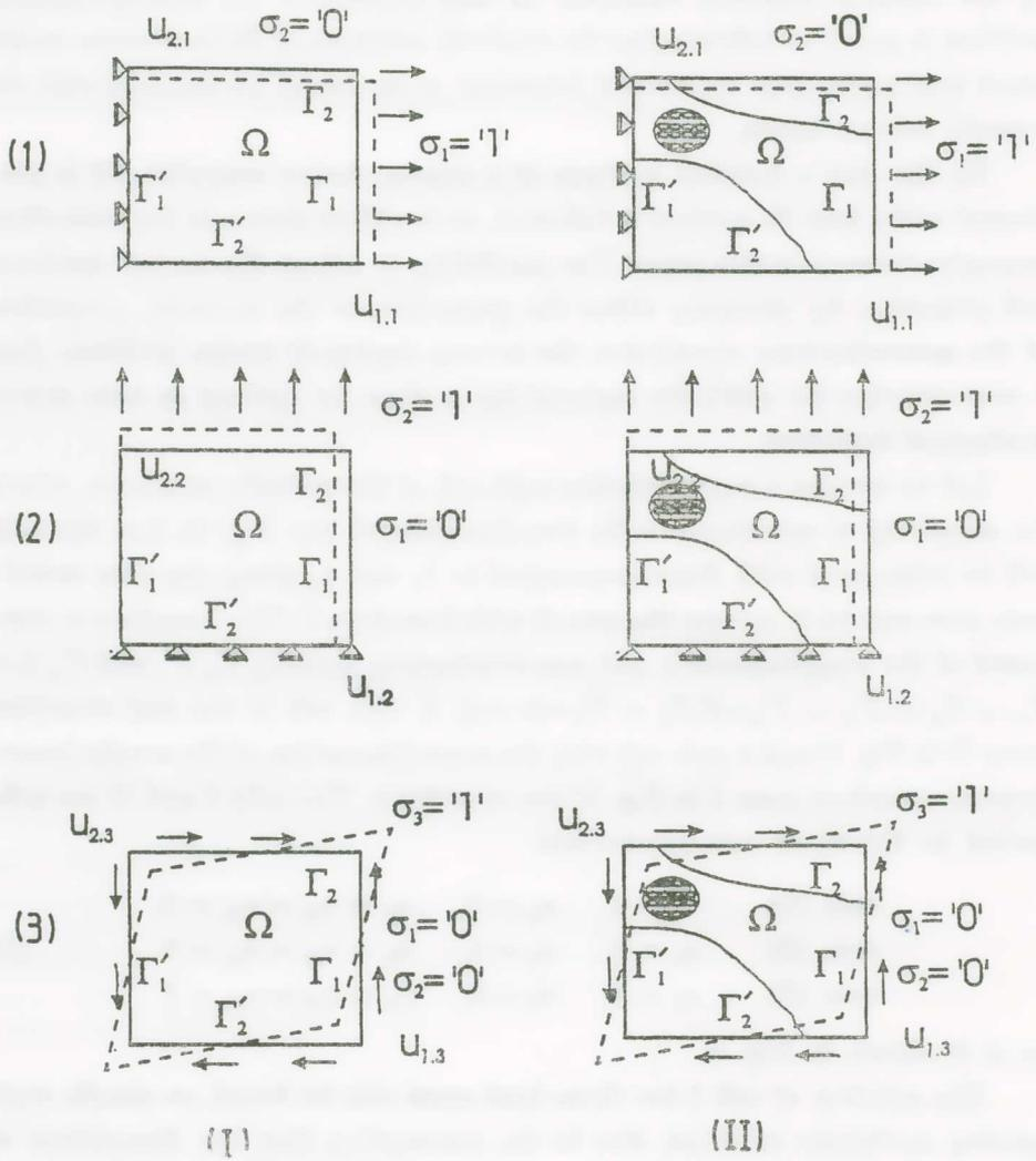
Fig. 1. Elements of the numerical homogenization technique for a unit-cell. Case (I) the homogeneous cell. case (II) the real structure cell. Problems (1) (2) and (3) indicate loading modes of the respective cells.
