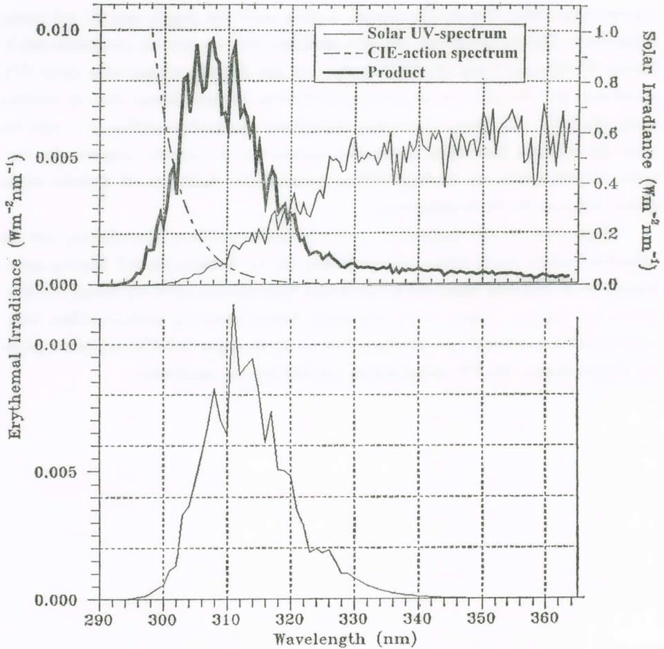
Fig. A2. Upper panel: the CIE-action spectrum (dashed line), a measured solar UV-spectrum (solid line), and the product of the two (erythema irradiance, heavy line). (From Kuik and Kelder, 1994). Lower panel: the response function of the YES UVB-1 pyranometer with the measured solar UV-spectrum of the upper panel.
