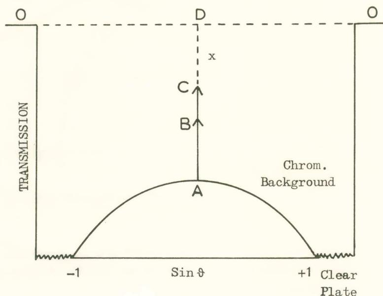
Fig. 4. Correction of the error due to mechanical inertia of the microphotometer.
